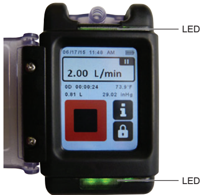
Figure 5. Green, flashing = Pump or schedule running
